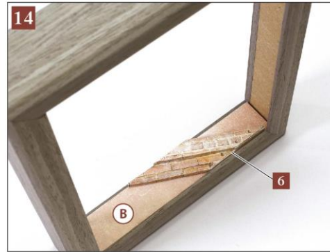
Paste 6 on the part B temporarily.
